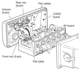
③ Install an optional unit to J3 on the AF board as shown below
