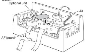
4 Reconnect the cables, and reassemble the unit to its original configuration.
