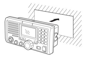
3 Attach the 2 supplied bolts (M5  $\times$  8 mm) on either side of the IC-M604A.
