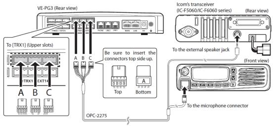
• The [TRX1] and [TRX2] ports (upper slots) accept the OPC-2275 connectors, however, follow the example to correctly connect the transceiver to ONLY the [TRX1] on the VE-PG3.
